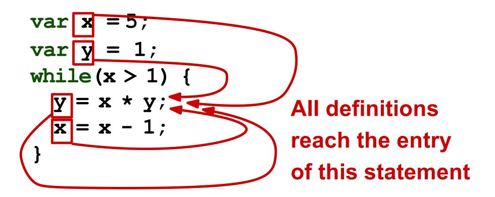
A reaching definition for a given instruction is an earlier instruction whose *target variable* can reach (be assigned to) the given one without an intervening assignment.
